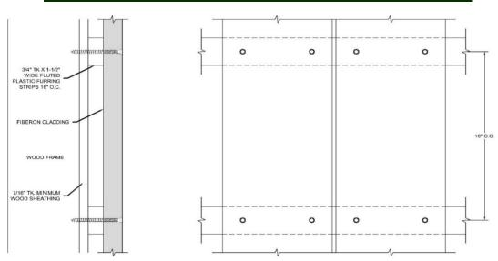
Figure 7 - Fastening Illustration only- open-joint Diagonal Application
