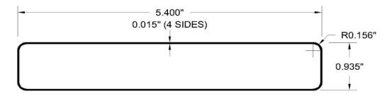
Figure 2 - Fiberon Wildwood Cladding (1x6, 1x8 & 1x12) and Concordia Cladding (1x8 & 1x12)
